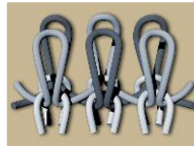
Interlock knitted structure
