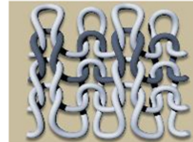
Rib knitted structure
